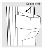
CAUTION: On models with an ice chute inside the top freezer door bin, be careful when placing items in the bin. Make sure that items do not block or fall into the ice chute.
